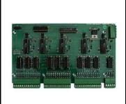
Dimmer output board to expand the number of analog outputs on the PROJECT central unit. Two extra boards of these can be connected on top of the basic unit which is default. Maximium 120 dimmer outputs are available this way.
