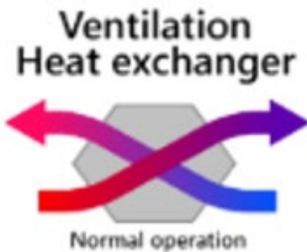
If you use a heat-recovery ventilation system instead, the energy loss will be limited to 10 to 20% instead of 100%. It not only results in a more sustainable solution but also in higher comfort and the HVAC system can be of a much lower capacity and will take a lower maintenance cost.
