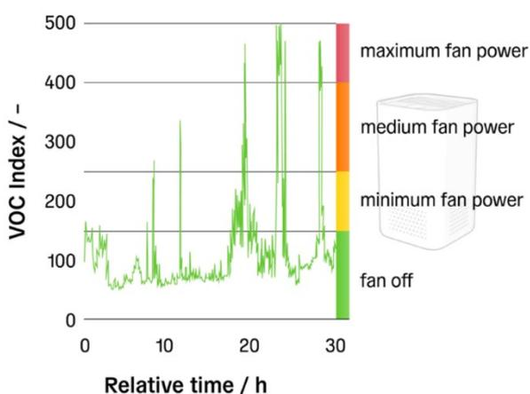
us if the concentration of one odour is truly higher than the concentration of another. Therefore, the VOC Index adapts its gain according to the VOC events of the past 24-hours learning time, leading to different VOC conditions being quantified on the same limited scale: a VOC Index ranging from 1 to 500. In this way, one can use a
