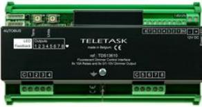
The TDS13610 fluorescent dimmer interface has 8 analog 1-10V outputs to control dimmable fluorescent lights. The interface also provides the necessary 8 output contacts to switch the main power supply to the 8 dimmed light units.
