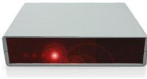
Residential multi-room/multi-source (MR) audio/video systems are often still provided with an RS232 control interface. Besides the existing wide range of audio/video integration solutions, TELETASK therefore introduces a configurable and learnable RS232 audio/video interface.
