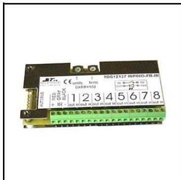
Interface with feedback to be connected on the AUTOBUS. This interface has 8 voltage free contact inputs. These are to be used to connect for example push buttons (any brand), window contacts, etc.
