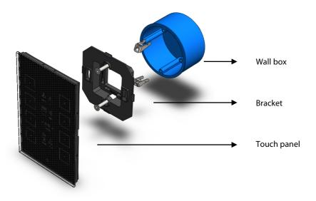
The design of the AURUS-OLED enables you to place the touch panel both vertical as horizontal. The choice is up to you or your customer!
