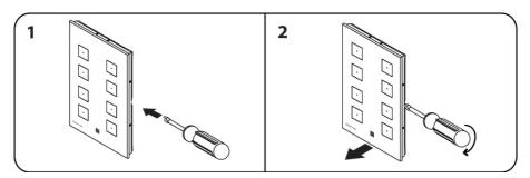
To remove the AURUS-OLED out of his wall bracket, place a flat screw driver into the holes at the sides of the AURUS-OLED. The wall bracket is provided with two clips which protect the wall during this action! Do not remove the AURUS-OLED by pulling the glass front panel, or warranty will void.
