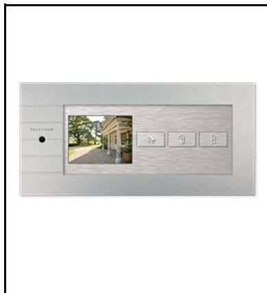
The LATUS Monitor touch window works as a discrete quality colour monitor to be connected with up to two video cameras.
