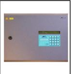
32 internal input (externally expandable up to 192) and 2 internal inputs for analog sensors (expandable to 10). 24 relay outputs 250V/10A, which can be extended externally with 16 relays 2A/250V plus 56 (7 x 8) relays on AUTOBUS 16A/250V = 96 relays in total. 50 powerful programmable clocks (actions) are available. They can take actions every x- days, weeks, months, years, only on weekends, working days, etc...
