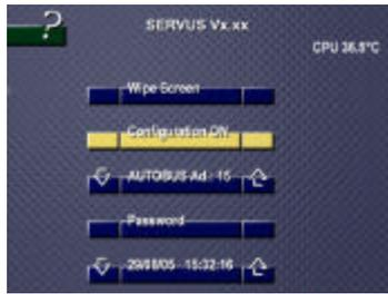
When the configuration button is in the ON status it is coloured yellow and there are more extra buttons available on the configuration screen. Beside of this, in some of the other screens, red coloured buttons will appear to be able to alter the user settings. For example in the sensor screens, there will be extra (red) buttons to be able to change the temperature presets for day, stand-by and night temperature settings.
