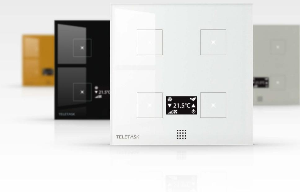
The built-in temperature sensor is used to measure and manage the room temperature. No extra thermostat needed anymore. AURUS-TEMP all and more capabilities on board.
