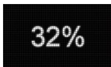
**Air humidity percentage** can be displayed by a second click on the upper-central hidden button (see drawing). It's a percentage of relative air humidity in the direct surroundings of the touch panel (the sensor is built-in in the panel).
