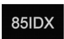
**The VOC index (air quality index)** can be displayed by a third click on the upper-central hidden button (see drawing). The following values are interesting to know since your ventilation system is most likely pre-configured by your system integrator:
